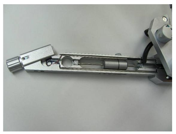
In this SA-1 photo above, you may notice two small metallic round tubes, running the underside of the arm wand, along each side. This separates the right and left channel signals from the phono cartridge in order to produce optimal channel separation.
