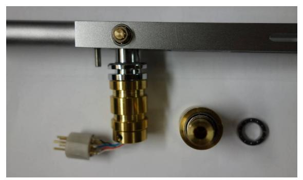
In this SA-1 assembly photo, two sets of fine miniature bearings, of the "rolling element bearing" type, are installed for both horizontal (set in bearing stem column in this photo) and vertical (further small bearing at left side of tonearm wand). This assures audiophiles of smooth tonearm function, greater longevity and consistency, and the ability to track warped vinyl.
