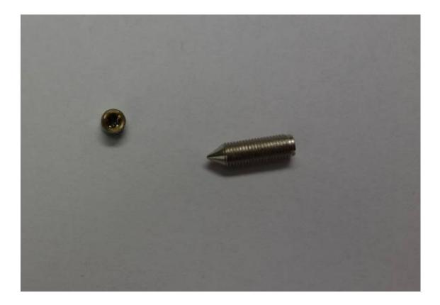
The same type "rolling element bearing" used in the SA-1 for horizontal movement is also used for the TA-1, while a delicate pivot bearing is applied for vertical movement (this is still a bearing but the bearing axis end is cone shaped, and requires careful assembly and adjustment). The right side cone in this photo is inserted into the miniature bearing inner race.
